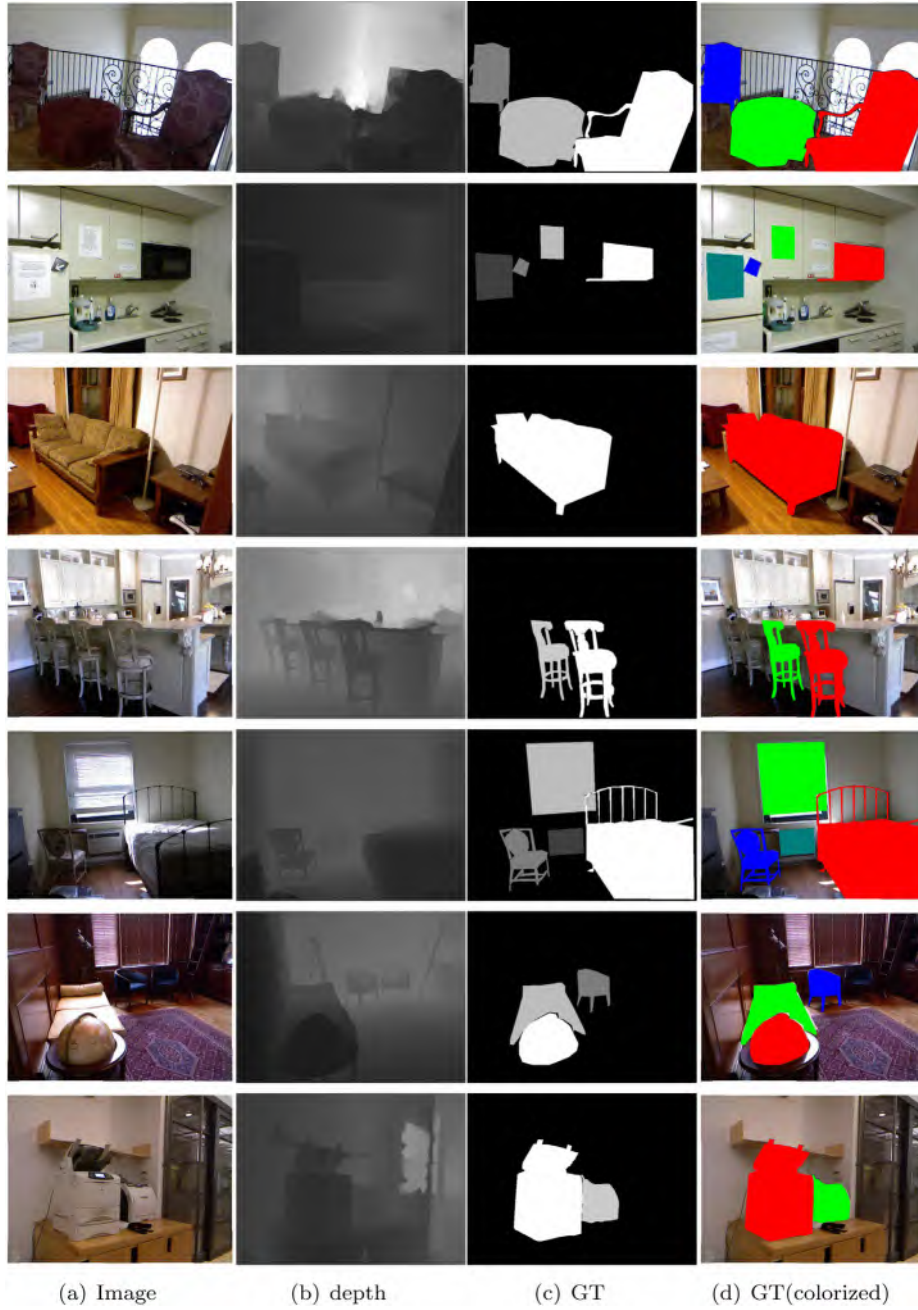
Fig. 1. (a) Image from our dataset, (b) corresponding depth map, (c) corresponding ground truth(GT) for saliency rank and (d) corresponding GT for saliency rank (colorised, red represents for rank 1, green represents for rank 2, blue represents for rank 3 and cyan represents for rank 4+). (For interpretation of the references to color in this figure legend, the reader is referred to the web version of this article.)
